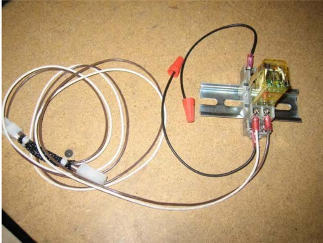
This relay harness plugs in between in between the gas valve and gas valve harness on the rear of the control panel under the oven. The relay provided is wired to operate as the ON/OFF switch for the exhaust fan. The relay closes when the oven is switched on which starts the exhaust fan.
